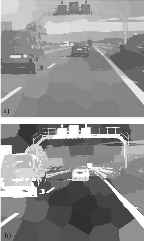
Fig. 4: Illustration of the measure for the reliability of trajectories. The result of clustering is shown in (a). The reliability measures for each cluster is shown in (b). Bright values indicate high reliability.
