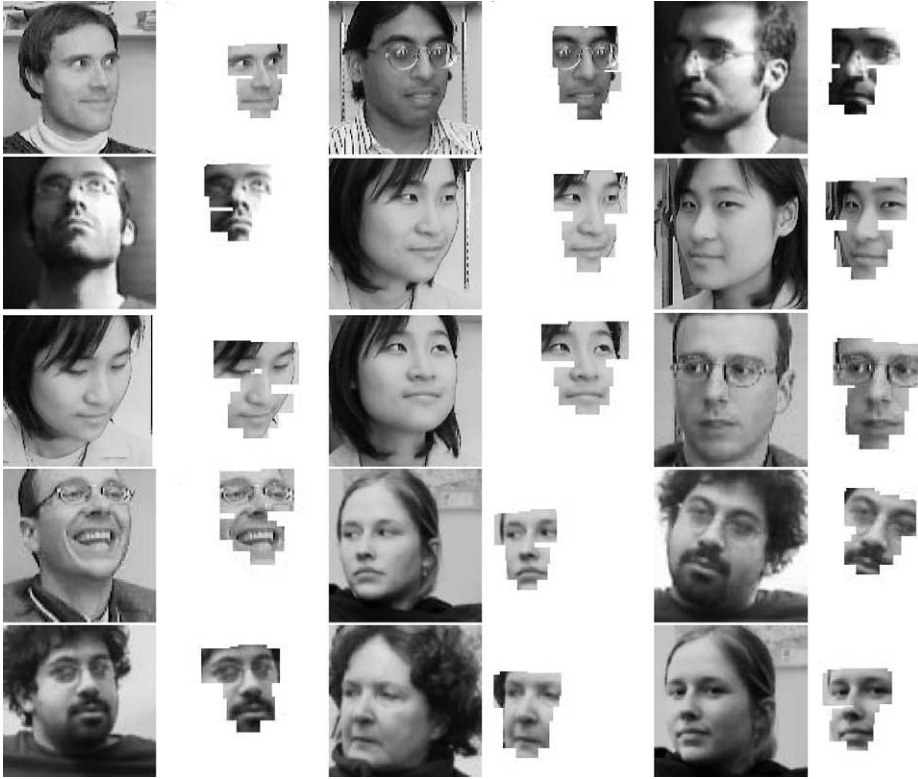
Fig. 6. Examples of component-based face detection. Shown are face parts covered by the 10 components that were used for face recognition.
