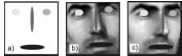
Fig. 4. Matching with a set of component templates. (a) The schematic component templates for a frontal face are shown. Shifting the component templates can compensate for slight rotations of the face in (b) the image plane and in (c) depth.
