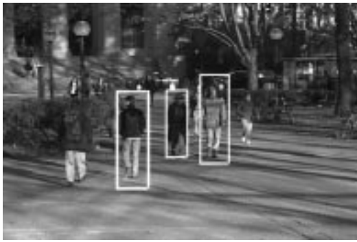
Fig. 2. Results of detecting people using Haar wavelets as inputs to an SVM classifier [24].
