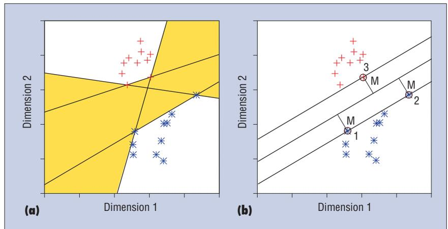
Figure 1. (a) The yellow area shows all possible hyperplanes that separate the two classes (represented by + and \*). (b) The optimal hyperplane maximizes the distance to the closest points. These points (1, 2, and 3) are support vectors. The distance  $M$  between the hyperplane and the SVs is called the *margin*.
