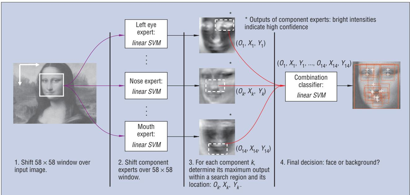
Figure 4. System overview of the component-based detection system.
