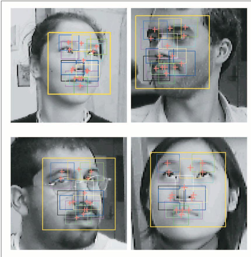
Figure 7. Faces detected by the 14-component system.
